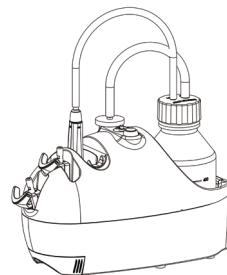
\*\* See Fig.2: Connect "LIQ" (Liquid inlet) to suction kit and connect "AIR" (air outlet) to vacuum source.
