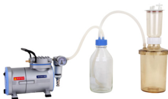
Using a safety bottle to prevent from overflowing
