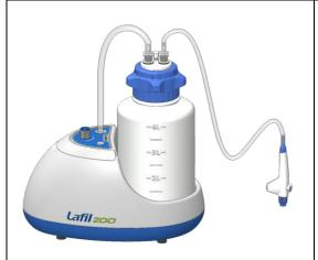
Assemble the short tube with the disc filter to the "AIR" hose barb of the suction cap.
