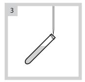
Hold vial at 45-degree angle. Add 2 ml sample to another COD reagent vial as the test sample.
