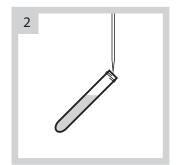
Hold vial at 45-degree angle. Add 2 ml pure water to one COD reagent vial as the blank sample.
