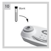
Insert the blank sample vial into CD 200 detector to start a zero calibration.
