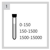
Select the appropriate concentration of reagent according to the COD concentration of sample.
