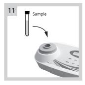
Insert the test sample vial into CD 200 detector to start a test.
