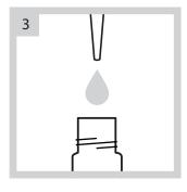
Add 5 ml pure water to one reagent vial as the blank sample.
