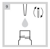
Add 2 ml of 1.54N Sodium Hydroxide Standard Solution to each vial. Close the vials and invert to mix.
