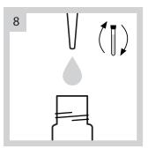
Add 2 ml of 1.54N Sodium Hydroxide Standard Solution to the vial. Close the vial and invert to mix.
