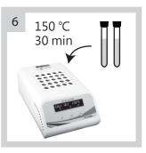
Put the vials into CR 25 reactor then start to countdown from 30 mins at 150°C.
