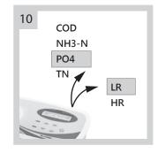
Turn on WD 100 colorimeter, then select test item and concentration range.
