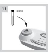
Insert the vial into WD 100 colorimeter to start a zero calibration.
