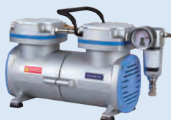
Rocker 910 Max. vacuum : 25 mbar abs. Max. flow rate : 55 (45) L/min
