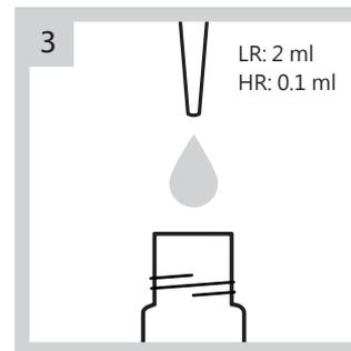
Add sample to another reagent vial as the test sample. Adding volume is as below: LR: 2 ml, HR: 0.1 ml.
