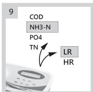
Turn on WD 100 colorimeter, then select test item and concentration range.
