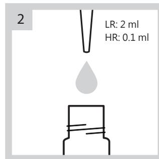
Add pure water to one reagent vial as the blank sample. Adding volume is as below: LR: 2 ml, HR: 0.1 ml.
