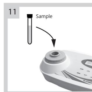
Insert the test sample vial into WD 100 colorimeter to start a test.
