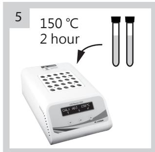
Put vials into CR 25, COD reactor then start COD program to heat at 150°C for 2 hours.
