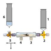
Detach the syringe contaning the recovered particles from the nozzle 6 and collect into a clean tube.
